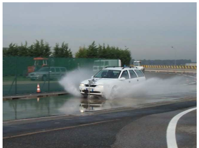
Fig. 2: Configured as shown, the small amount of spray entering the sensor field of view has no effect on measurement accuracy.
