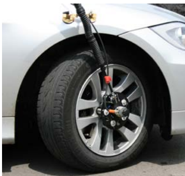
Fig. 2: WPT sensor mounted at the front wheel
