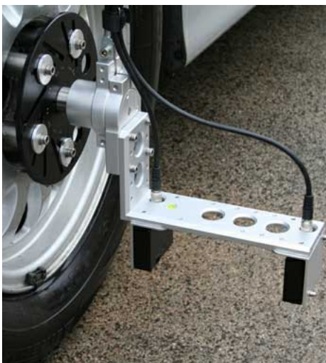
Figure 7. The new CORRSYS-DATRON Dynamic Camber Angle Measurement System acquires dynamic wheel camber values by comparing the relative change in height between two HT-250 Sensors.
