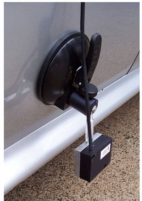
The CORRSYS-DATRON HT-250 Sensor uses laser triangulation technology to measure dynamic vehicle ride height.
