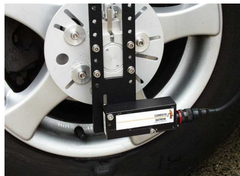
The CORREVIT® SF II P Sensor enables simultaneous measurement of longitudinal, transversal and magnitude speed, as well as angle.
