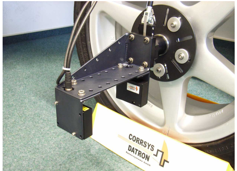
The new CORRSYS-DATRON Dynamic Camber Angle Measurement System acquires dynamic wheel camber values by comparing the relative change in height between two HT-250 Sensors.
