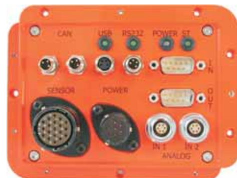
Fig. 2: Electronics unit of the Corrsys-Datron Microstar II sensor
